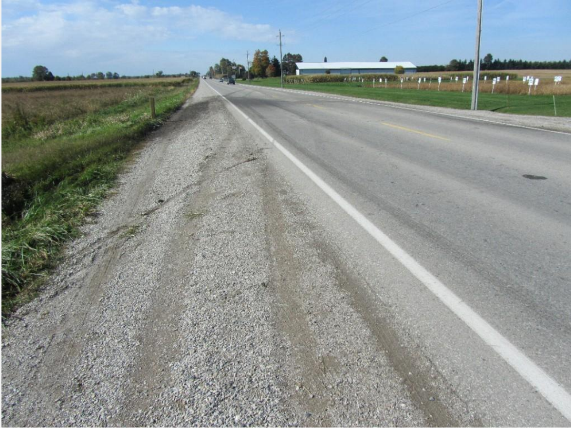
View of the yaw marks heading back toward the road surface as the loss-of-control vehicle continues to rotate clockwise.
